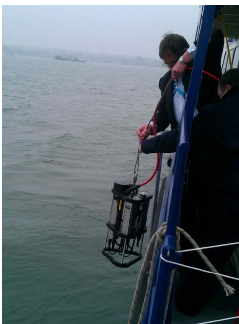
Deployment of fluorescence water quality analyser (Chelsea Technologies Group 2018)
